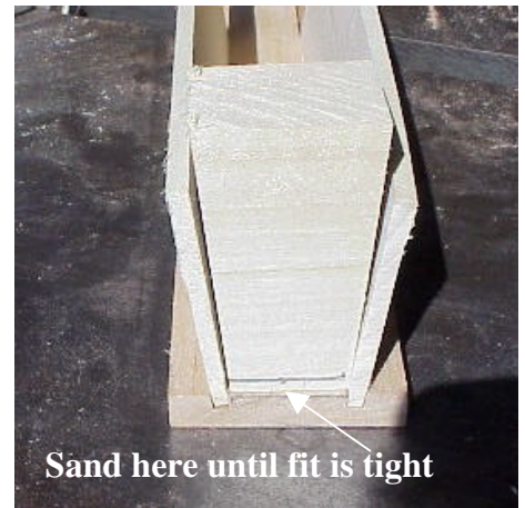
Test fitting the end blocks
