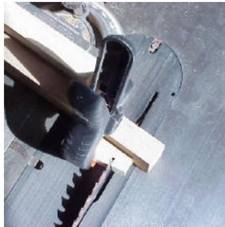
Trimming bottom of blocks
